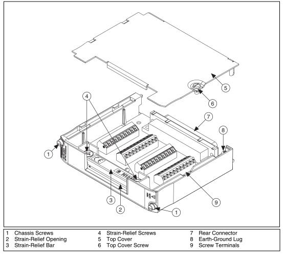
Figure 1. PXI-2621 Parts Locator Diagram
