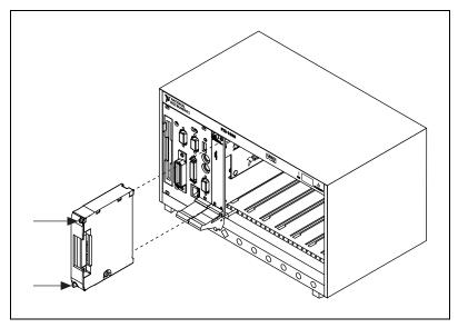
Figure 2. Connecting the TB-2621 to a PXI Module
